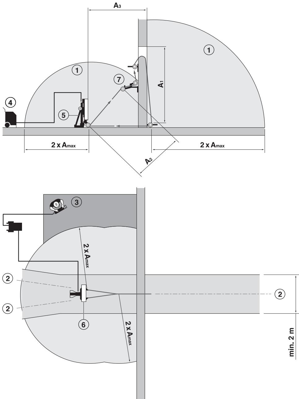
(A<sub>max</sub>) Largest free running wire section (A<sub>1</sub>-A<sub>3</sub>)
