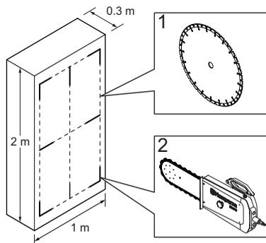
Feed the blade 3-7 cm (1.2"-2.8"). Make the pilot cut in order to obtain a straight cut and with that a base for the next cut. The cut should be made with care. The cutting arm allows blades up to 1000 mm (40") to be used as the start blade. It is, however, recommended to start cutting with a 800 mm (31.5") blade.
