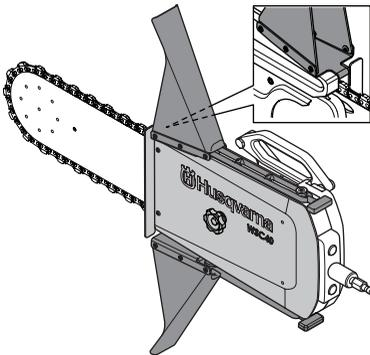
The cover and spray guard provide protection against contact with moving parts, ejected debris, thrown water and concrete slurry. The spray guards are also designed to catch the diamond chain if it snaps or jump off.
