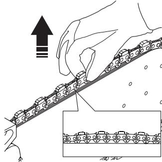
Loosen the screw for the clamping washer from behind using a 13mm t-box spanner. Use the adjustment knob to tension the chain.
