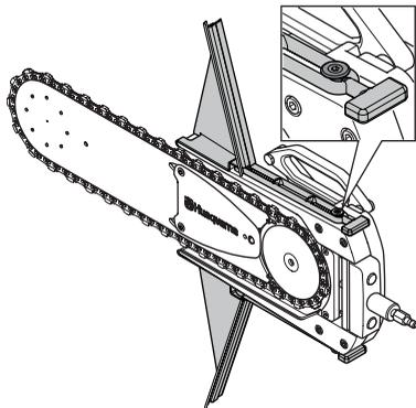
We recommend that both flush guards are fitted but in some applications (sawing aligned to the floor or the ceiling) one guard might be temporarily removed. At least the guard in the chain direction must be fitted. Replace the guard after cutting.
