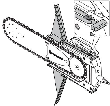
Check the guards for damages or wear. Ensure there are no damages on the guards. Replace the guards if damaged.
