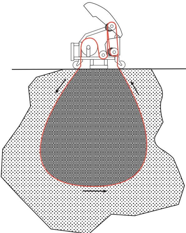
It may be necessary to drill holes to thread the wire through the material to be cut.
