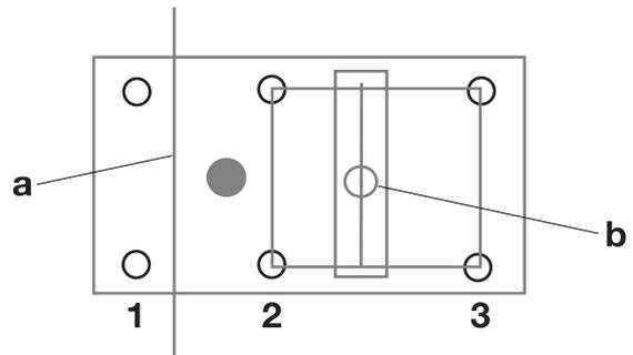
If necessary, fit idler wheels to assist the cutting process. Using the idler wheels allows the number of sharp corners that the wire must be pulled around can be reduced, which results in less wear to the wire at the same time as cutting is made easier. Using the idler wheels also lets the wire be guided in different directions without the need of moving the saw unit.
