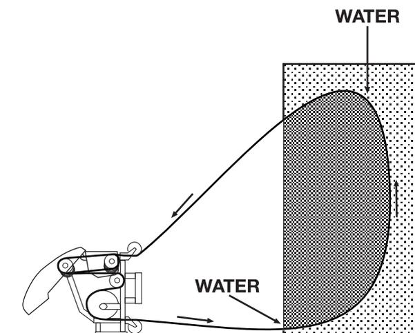
In addition to the cooling water from the water spear, the wire is rinsed by the two swivel wheels on the machine. This is to keep the wire as clean as possible, which means that the saw can work with less friction losses and greater efficiency as the wire becomes cleaner.
