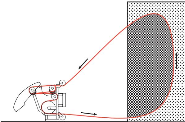
The saw is assembled horizontally when the cut is to be made at floor height and when the cut is made in the floor.
