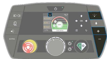
Switch off the Mist Cooler System by pressing the Mist Cooler System button on the control panel. See Control panel (HMI) page 22 position 8.
