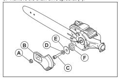
7. Install a new chain drive sprocket.
