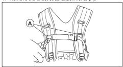
2. Attach the new chest strap (B) on the shoulder straps of the harness. Start with the lower part of the chest strap attachment (A).
