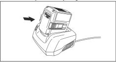
Make sure that the green charging light on the battery charger comes on. That means that the battery is connected correctly to the battery charger.
