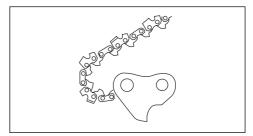
774 - 006 - 19.09.2023 19  Bar groove width, in/mm. The groove width in guide bar must be the same as the chain drive links width.
