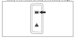
When all LEDs on the battery come on, the battery is fully charged.
