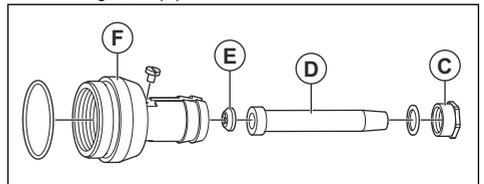
**Note:** The nut (C) has a right hand thread.
