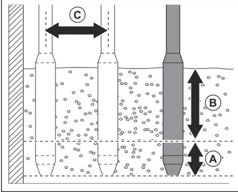
3. Wait approximately 10–20 seconds until the surface around the vibrator head is shiny and no air bubbles come to the surface.
