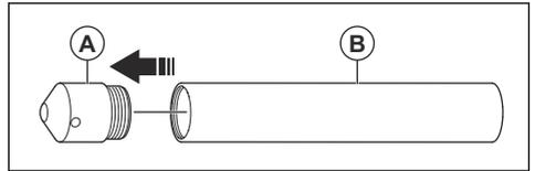
**Note:** The end cap (A) has a right hand thread.
