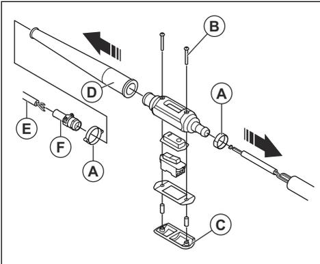
2. Remove the screws (B), remove the switch box cover and disconnect all wires from the switch.
