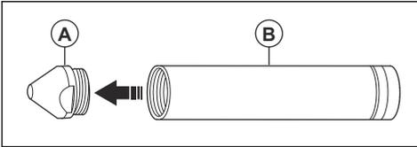
**Note:** The end cap (A) has a right hand thread.
