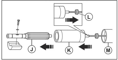
4. Use an applicable rod and a hammer to carefully push each part through the stator tube (M).
