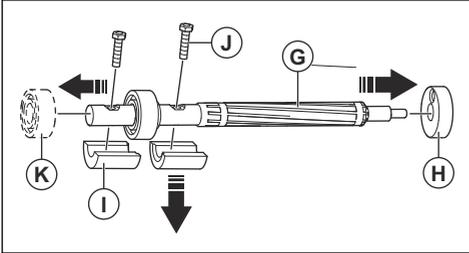
5. Remove the bearing holder (H), the eccentric element (I) and the screws (J).
