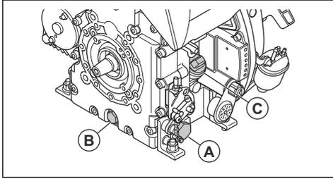
2. Remove the oil drain plug (A) or (B) and connect a hose.
