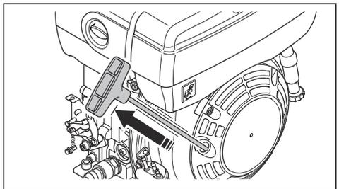
3. Release the starter rope handle to let the starter rope go back.
