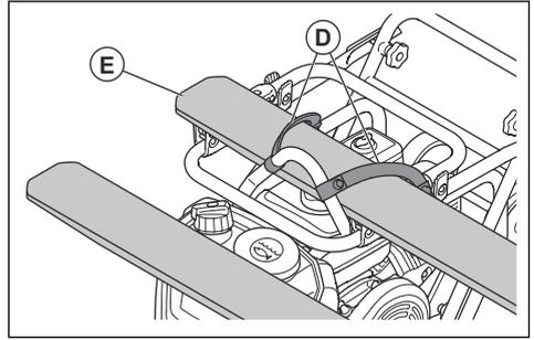
**Note:** The straps are standard equipment on model LF 130 but optional on models LF 75, LF 80, LF 100
