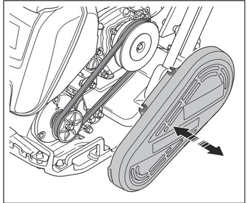
3. Examine the V-belt for damages and wear. Replace the V-belt if it is necessary.
