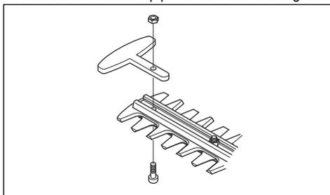
2. Assemble the screw and the nut to the cutting unit and tighten to 8 Nm.
