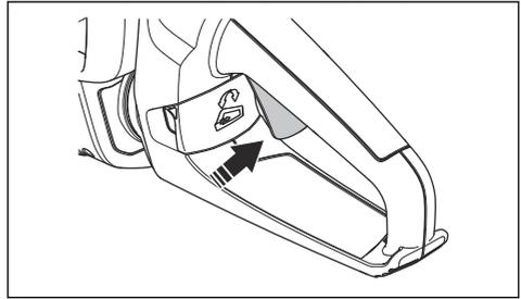
4. Release the power trigger and make sure that the return spring operates correctly. The blade must stop in less than 1 second.
